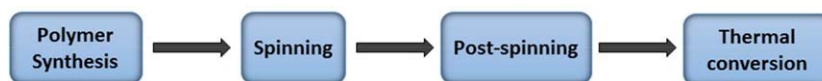
Figure 1. Stages of carbon fiber manufacturing. [Color figure can be viewed in the online issue, which is available at wileyonlinelibrary.com .]
